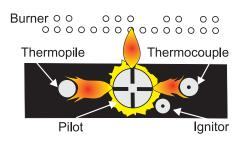
Periodically check the pilot flames. Correct flame pattern has three strong blue flames: 1 flowing around the thermopile, 1 around the thermocouple and 1 flowing across the burner (it does not have to be touching the burner).
